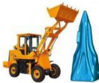
Digitization of 3D scanning of shovel teeth
